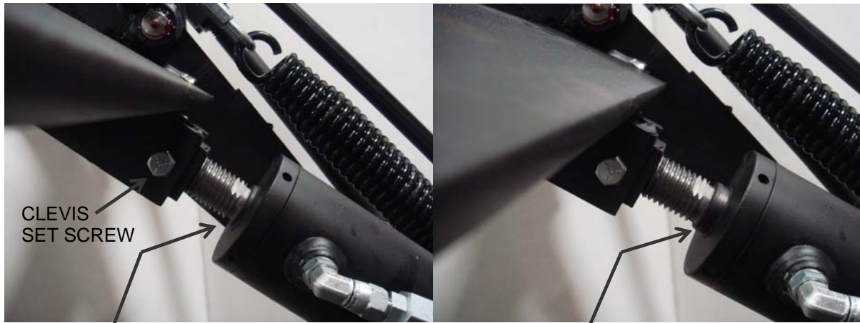
CYL ROD RETRACTED, DO NOT FORCE TRUNNION TUBE LOWER
