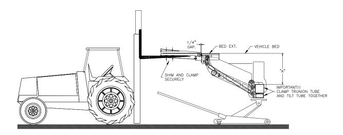
Next raise the gate Trunion Tube using one floor jack in the center. Hold the "A" dimension in the range given on Page 3. The face of the Trunion Tube must be square to the vehicle bed and the primary platform must be even with the Bed Extension across the entire length.
