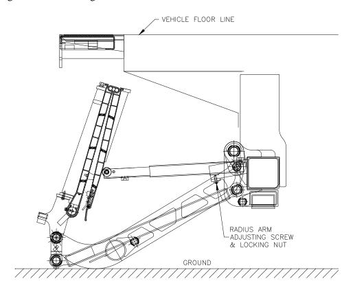
The higher the Radius Arm is adjusted, the slower the platform will fold, and more clearance at the frame rails will be required. But if the platform leans too much toward the front of the vehicle with the lifting arms on the ground, it will be harder to unfold. Radius Arm will pivot up when gate is folded, once the optional ICC bumper is installed. Ground clearance for the Radius Arm is not an issue.
