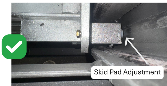
Good Skid Wear Pad Adjustment Correct pad adjustment: 3/16" from track
